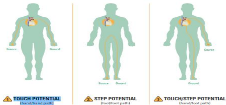
Figure 2.2: Illustrates the path of current through the body. Here are some rules, which should help you to avoid electricity hazards.
